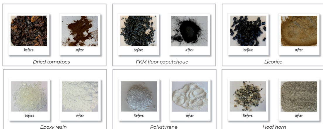
Figure 6: Different materials before and after grinding in the MM 500 control
