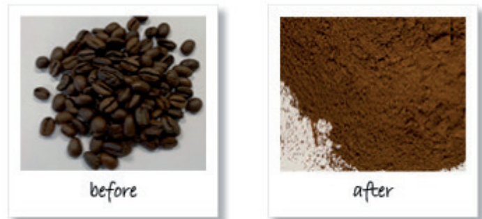
Figure 3: Left: Roasted coffee before and after grinding in the MM 500 control (per 125 ml stainless steel grinding jar: 5.4 g coffee, 8x20 mm stainless steel grinding balls), set temperature -100°C, 25 min pre-cooling time, grinding in 10 cycles (1 min 30 Hz + 0.5 min 5 Hz).
