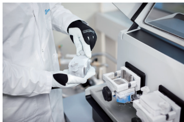
Figure 2: Deeply frozen grinding jars after cryogenic grinding with the MM 500 control
