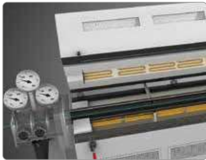
Interior view of custom designed FZS with flanges for inert gas counter flow for open operation during inert gas heat treatment
