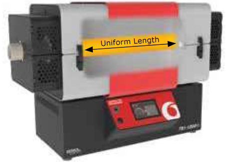
Carbolite Gero's design features optimised uniform zone
